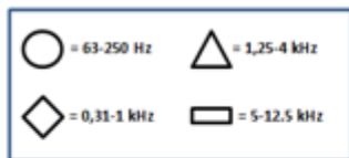
Fig. 3: Spectral range zones: geometrical code for frequency value notion in maps with amplitude on the Y axis. This code is used for spectral constellations. Source: own elaboration.
